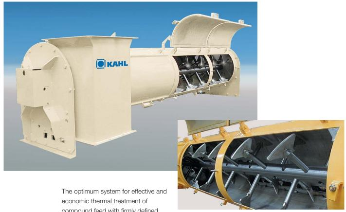
The optimum system for effective and economic thermal treatment of compound feed with firmly defined ratio of retention time and throughput. The MK is appropriate for the treatment of mash feed or as conditioner prior to the pelleting press.
