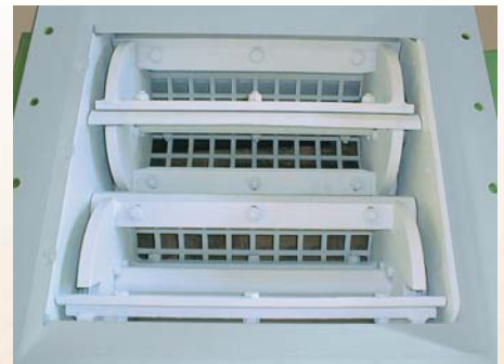
The particle size of the expanded product can be determined by means of the downstream crushing device.
