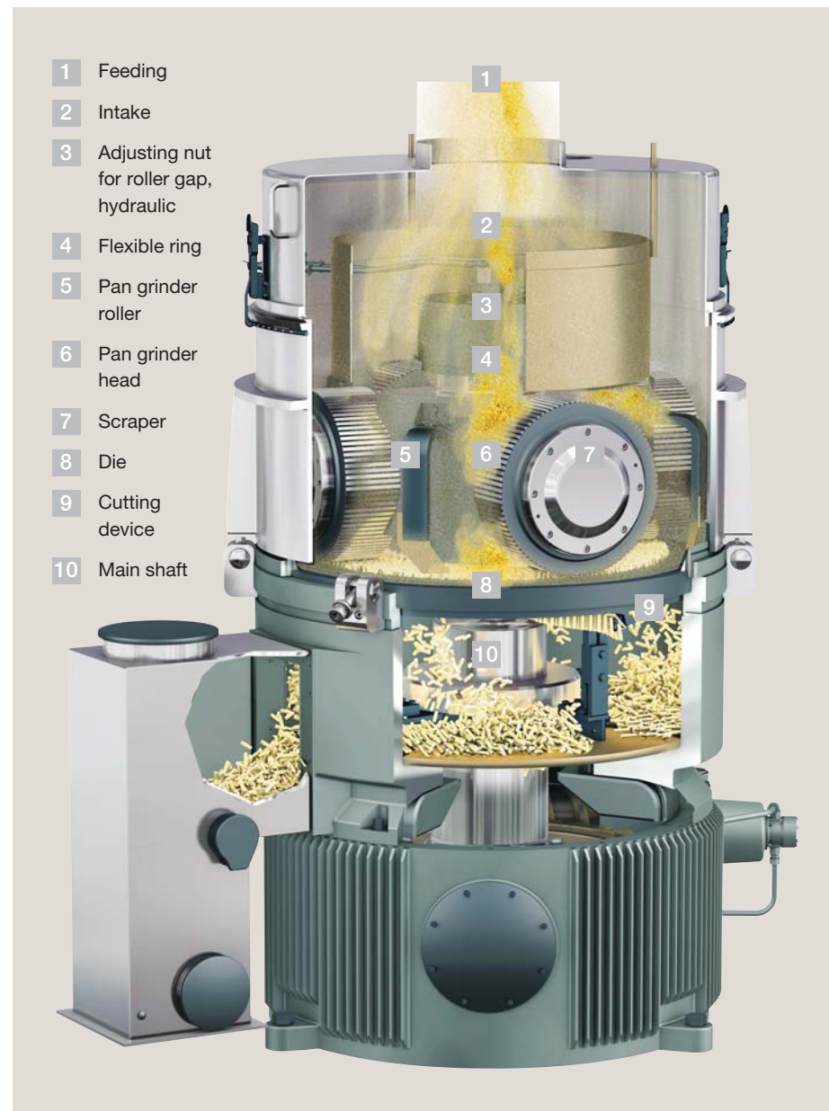
Fig. 1: Main parts of the flat die pelleting press:
