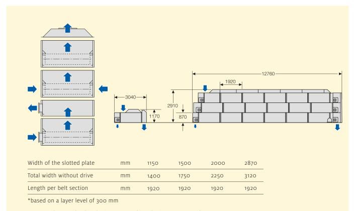
Intermediate aspiration for the separation of the process sections, e.g. pre-cooling and post-cooling, pre-drying and post-drying, drying and cooling.
