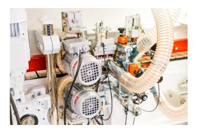
BUFFING UNIT 2 motors 0.05 kW, 1,500 rpm provide a super-finish for ABS and PVC edge material.
