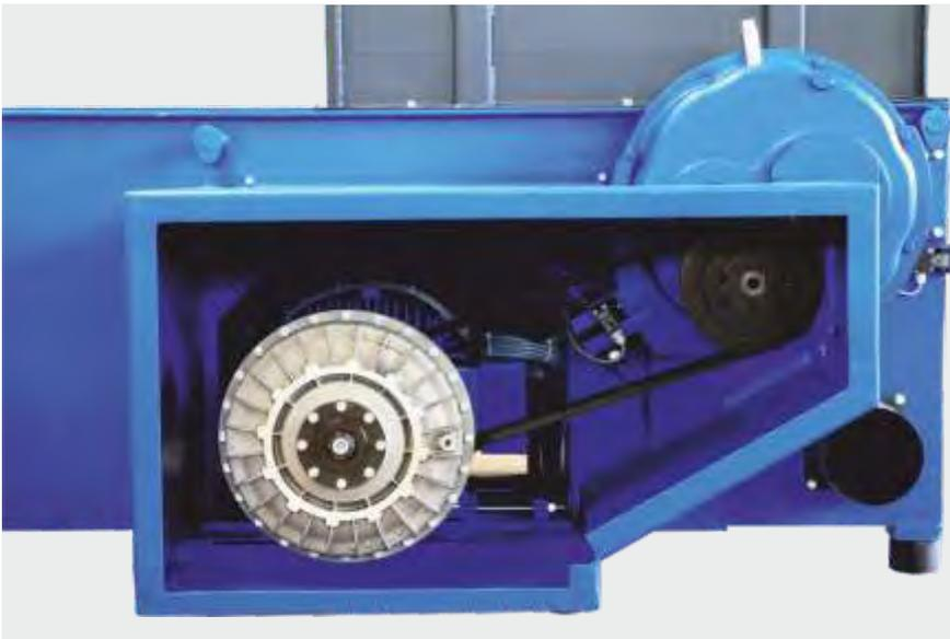
Powerful drives, with optional hydraulic clutch, 5-fan belts, robust gearbox, gear limit
